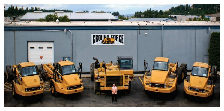
Ron Nilson, Ground Force Manufacturing, builds fuel and lube trucks for the mining industry based on Cat rigid- and articulated-frame chassis. Ground Force purchases Cat articulated- and rigidframe truck chassis as the base for its line of fuel and lube trucks, water trucks and cable reel trucks. Diesel fuel capacities of Ground Force fuel and lube trucks, for example, range from 2,500 to 25,000 gallons.
