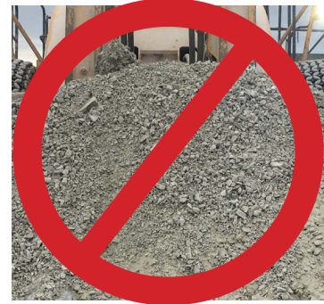
INCORRECT MATERIAL: Too small, full of fines, and not screened.
