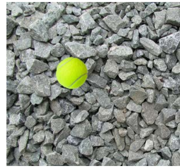
PREFERRED MATERIAL: Two-inch (50mm) minus, screened, and washed gravel
