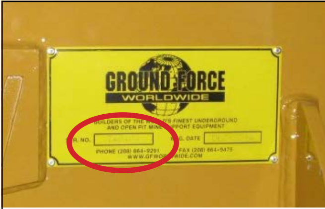
Located on the driver side or in quick fill or in electrical box. This plate will be found on all Ground Force equipment from 2007 to current.
