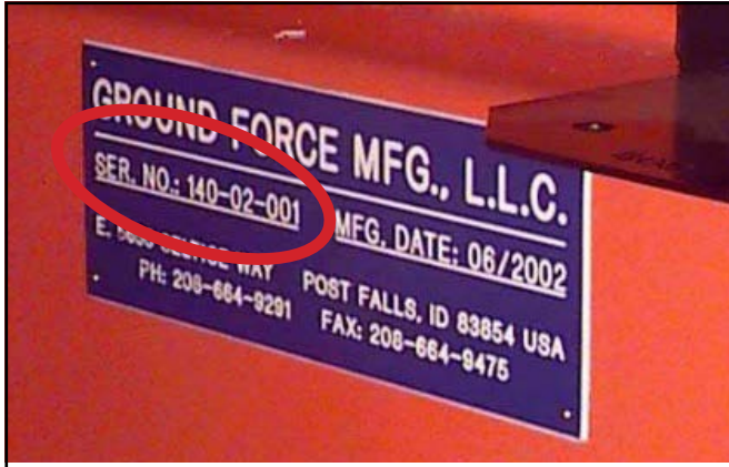
Located on the driver side of trucks. This plate will be found on all Ground Force and ARESKO equipment from 1985 to current.
