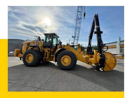
Ground Force Cable Reeler Attachments are designed to work with most loaders and dozers for the safest and most efficient electric cable placement in the industry today.
