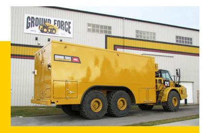
Ground Force Lube Only Bodies offer maximum capacities of lubrication when your operation is large and you need efficient delivery of fluids. These bodies are engineered to fit rigid frame, articulated, and conventional chassis to offer the most diverse fleet lineup.
